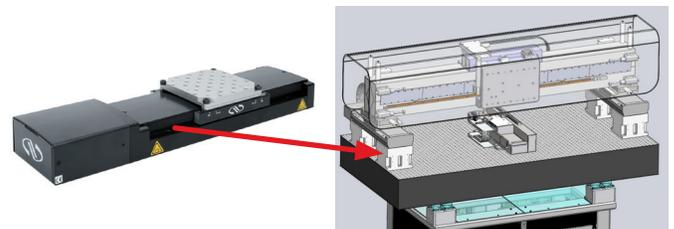
Bridge is often mounted in Gantry-Architecture and Moved by Linear Translation Stages
