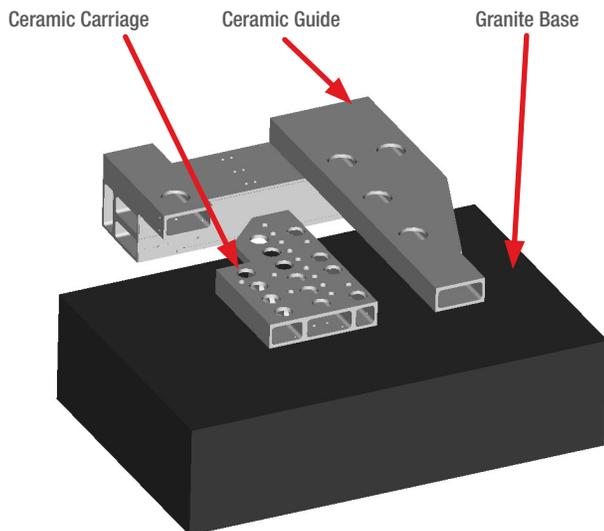
*Clean and Simple Architecture of DynamYX includes Three Monolithic Elements*
