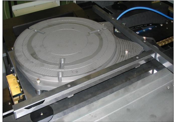
Ceramic Chuck with Integrated SiC Mirrors
