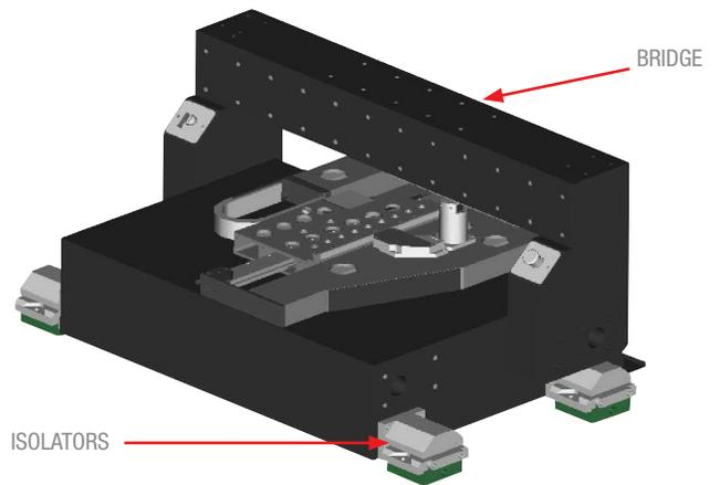
A Typical DynamYX 300 System is comprised of a granite base which serves as the reference surface for the XY air bearing carriage, the moving stage elements, an overhead bridge structure for installation of an optical system, and a set of vibration isolators.
