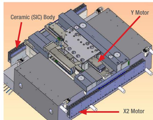
Three Linear Motors Drive the DynamYX and Datum Stage
