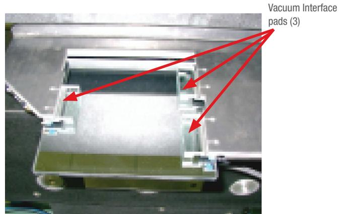
*The ceramic reticle holder of the RS stage provides a vacuum-secured 3-point mask interface which is ESD safe. This mounting plane has a very tight parallelism tolerance with respect to the axes of travel.*
