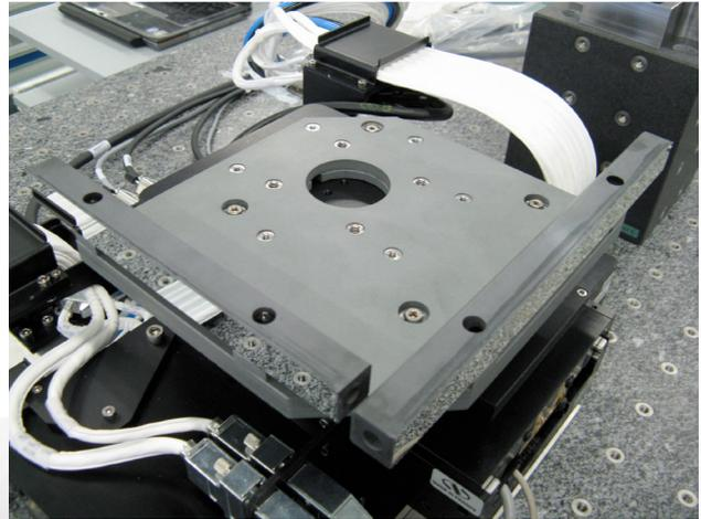
Ceramic plate with integrated (replica) interferometer mirrors on Newport XML crossed roller bearing stages can provide 50 nm XY bidirectional repeatability (when used with XPS controller and Renishaw interferometer).
